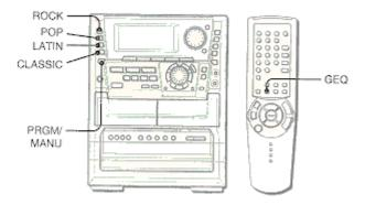
This unit provides four different programmed equalization curves.
