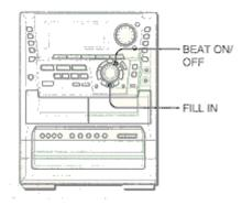
During playback with the BEAT function switched on, press **FILL IN** at the desired moment.
