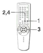
This unit is whumped with a built-in test signal generator called a noise sequencer for easy balance adjustment of all five channels. The sequencer outputs a noise signal that "travels" from channel to channel, enabling the simple adjustment of sound level to achieve, at the listening position, the same apparent loudness from each channel.
