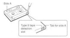
To record on the tape again, cover the tab openings with adhesive tape, etc. (On Type II tapes, take care not to cover the Type II tape detection slot.)
