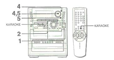
Two microphones (not supplied) can be connected to this unit, allowing you to sing along to music sources. Use microphones with mini plugs  $(\emptyset 3.5 \text{ mm}, 1/8 \text{ inch})$ .
